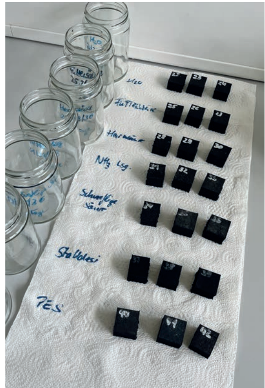
Figure 4: Test sample after acid resistance test
