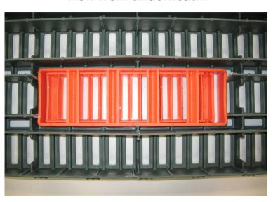
Press the manure flap against the slat and fix it with 4 Spax bolts 3,5x20 mm.
